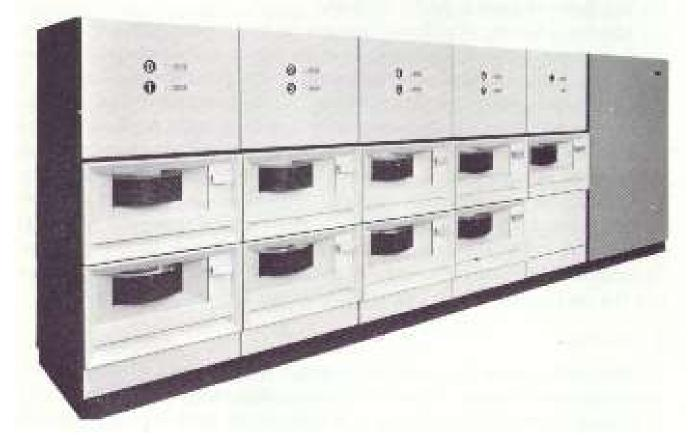
IBM 2314 About the size of 6 refrigerators 8 x 29MB (M!) Required similarsized air condx!
